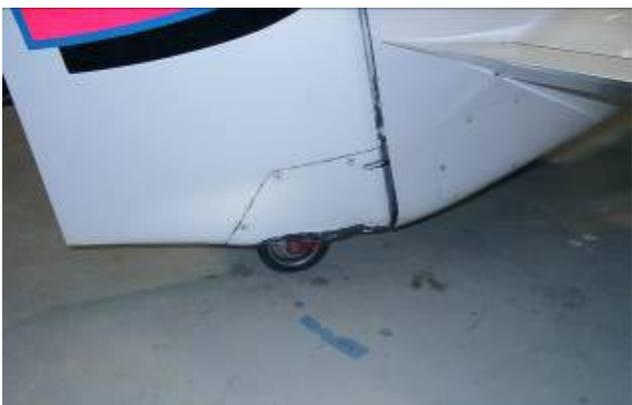
The tailwheel is cleverly buried in the rudder. The tailwheel is not supported by the rudder but turns with it at an exact 1:1 ratio
