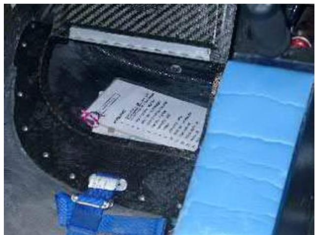
Secret checklist compartment under the pilot's knees. The pad on the center console is a critical part of the ingress-egress procedure, which includes stepping on the floor (also the seat bottom), sitting on the center console, swimming your feet under the panel, then sliding your hind quarters down into the seat.
