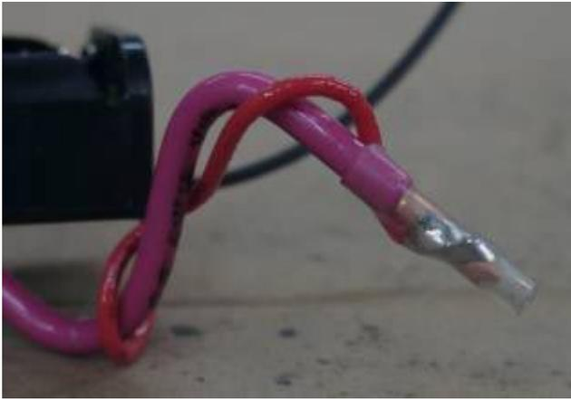
Cut the black wire from the battery holder as shown. Slip a piece of 1/16" heat shrink over the wire. Strip, attach, and solder the black wire to one of the terminals on the SPST switch. Be careful you don't shrink the heat shrink by accident while soldering the joint.
