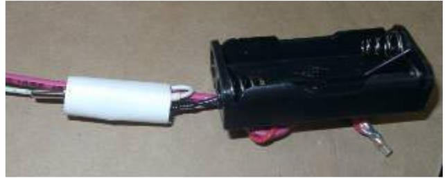
Shrink the heat shrink over the switch to hold the switch in place.
