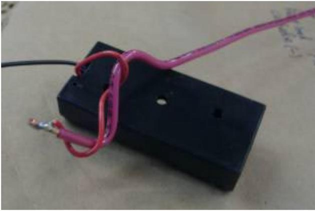
Optionally you can shrink a piece of 1/8" heat shrink over the joint, or just cover it with epoxy later. If you use heat shrink, be careful heating it, as the cheap insulation on the battery holder wire is not very tolerant of heat.
