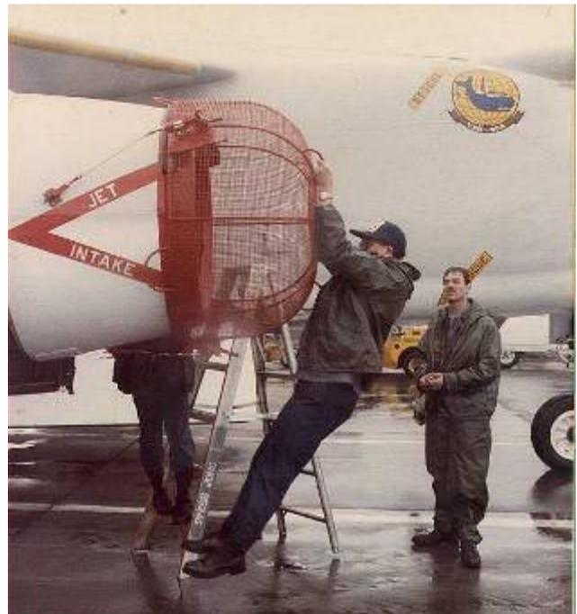
The objective was to design an engine inlet FOD screen that was less than 65 pounds and could be installed by one person. Also the screen could not restrict the engine airflow during ground runs at maximum thrust.
