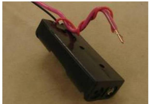
Solder the red battery holder wire to the 14 ga wire.
