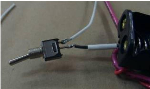
Slip a piece of 3/8" heat shrink over the wires and over the switch assembly as shown below.
