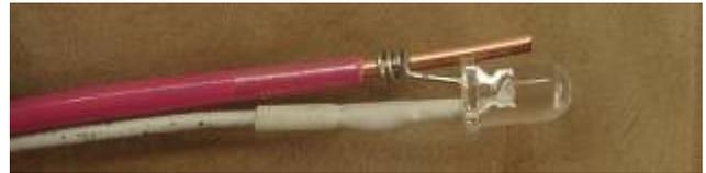
Solder the anode to the 14 ga wire.
