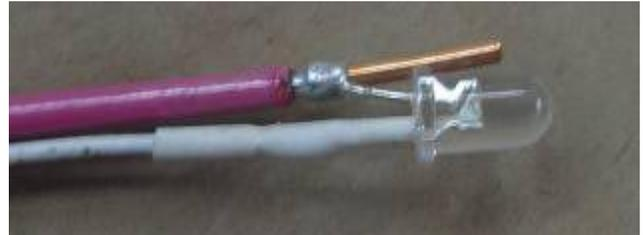
At the other end of the 14 ga wire, strip the end and bend it to a nominal "Z" shape. This shape will increase the torsional strength when it is epoxied to the battery box later. Wrap the red (positive) wire from the battery box around the 14 ga wire. Cut to length and strip the end as shown.
