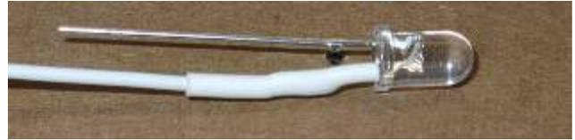
Take the piece of 14 ga solid house wire (the gauge is not critical—use what is available and sufficiently stiff) and cut it to the desired length, plus some extra to epoxy to the battery holder. Strip as shown below. Note the length and positioning of the stripped portion. This will be used to hold the LED in place. Wrap the anode (the terminal that you haven't used yet) of the LED around the 14 ga wire as shown below.
