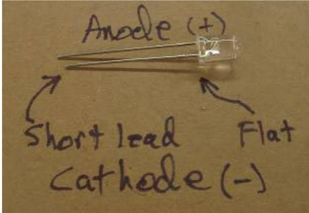
Shown above (before) is a picture that even I can understand. This is the LED listed in the parts list. The cathode is identified two ways. As it comes out of the bag, the cathode is shorter than the anode. Additionally, the cathode side of the plastic lens has a flat spot on it. If you're like me and can't remember what a cathode is, it's the side that connects to the negative (-) side of the power source. I guess it's a good thing I became an Aero Engineer instead of an EE.
