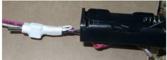
Slip several pieces of 1/4" heat shrink over the wire assembly. The last piece is shrunk over the LED as shown to hold the LED in place. The other pieces are shrunk to hold the 22 ga wire in place on the 14 ga wire.
