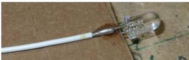
Slide the heat shrink tubing back up over the solder joint and shrink it with a hot air gun.
