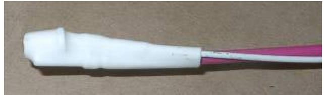
If necessary, trim the end of the heat shrink tube with a razor knife to expose the end of the LED.
