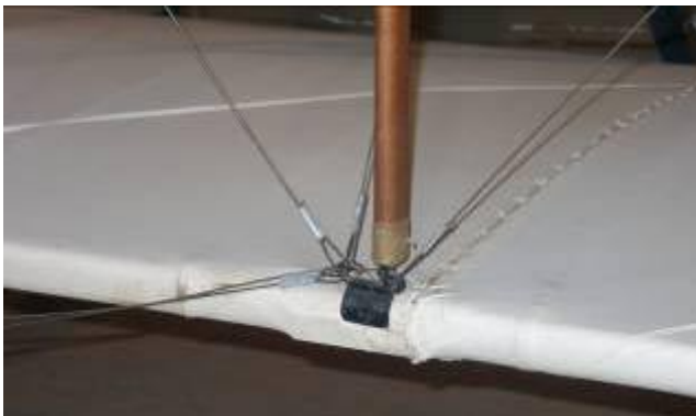
Strut on the Wright 1903 Flyer. Note the two hooks that make attaching struts and bracing wires quick and easy. This is typical of every connection on the airplane.
