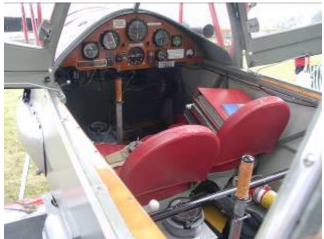
Where do you put the control sticks in a four place airplane? This Tiger Moth was modified after WWII, widened with two seats added. However, the control positions remained in tandem on the left side
