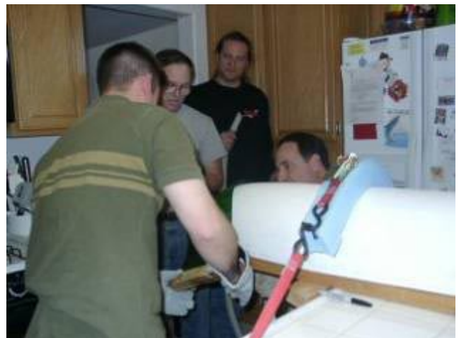
George "Knife" Gennuso and Cadet Nick Garasimowicz stretch the hot and floppy acrylic (Plexiglas®) over the nose of the wing tip
