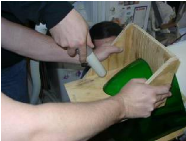
Ben Harvey directs the Reverse Vacuum Doofer onto the plastic to cool it
