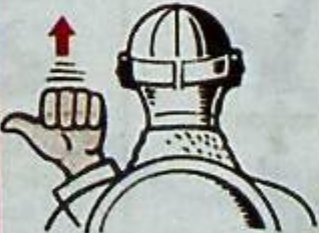
10. Upward Motion with Palm Toward Student Raise or Elevate Nose of Plane
