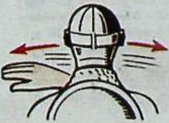
12. Hand, Palm Flat, in Sweeping Horizontal Motion Level Off or Maintain Altitude
