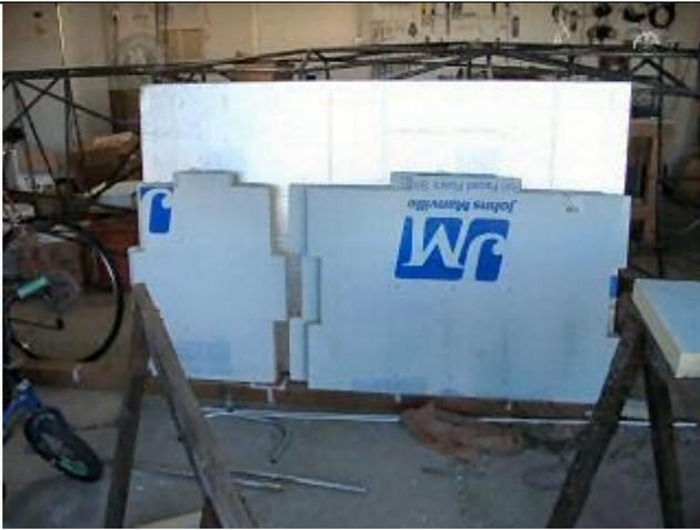
The material for the Hush Haus was simple 2" Foil-Faced Foam Sheathing. This was a yellow foam that I picked up at the local Home Depot. I needed two 4'x8' sheets, but had a bunch left over. I cut it with a simple crosscut hand saw (haven't used that in a while!).
