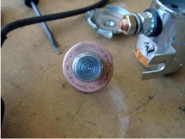
End on view of the plunger, showing noticeable pitting on the copper disk contact.
