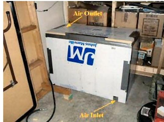
After taping the top on and placing over the compressor. A small hole (about 2"x2") was cut at the bottom and in the top to allow cooling air to move through by convection. The air outlet is at the opposite end of the box from the piston end of the compressor.
