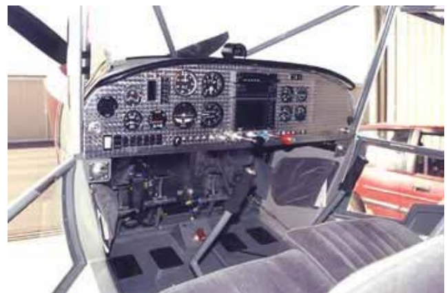
The entire instrument panel is machine turned and sprayed with clear lacquer
