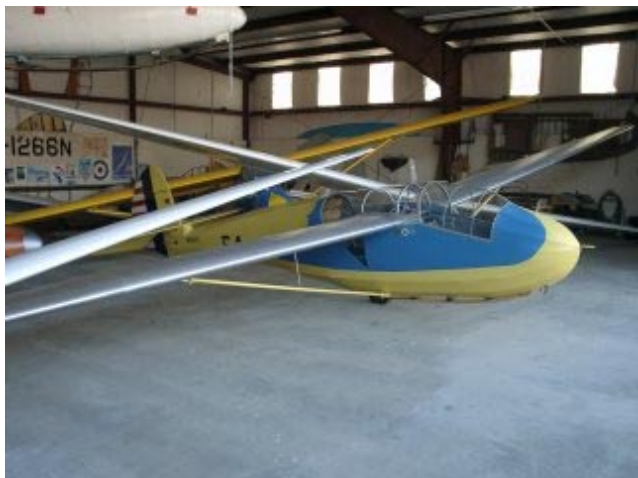
Schweizer TG-2 WWII training glider. Not a whole lot of these were produced, and this is one of the few left flying. Jeff restored this one from a basket case. The all metal wing is mostly constructed with PK screws with a few soft rivets
