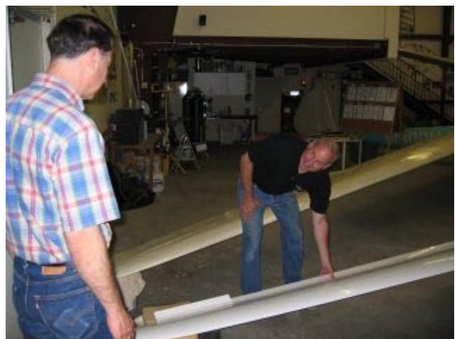
Jeff demonstrates the Genesis 2 drag flap to Vice Kommandant Gennuso. When the aileron deflects up, this flap deflects up at twice the rate, reducing the adverse yaw and thus reducing rudder usage
