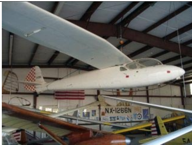
Condor IV built in Argentina from a German Schleicher kit in 1953. Jeff explained that the elephant ear rudder minimized twisting moments on the tail boom.
