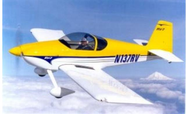
RV-7. It's pretty much a -9 fuselage (12" longer than a -6 with a little more head room), RV-8 wings and tail, except for the rudder, which is a -9 rudder. The original -7 rudder, which was basically an -8 rudder (also -6), didn't allow spin recovery quick enough, so Van's put a bigger rudder on it.
