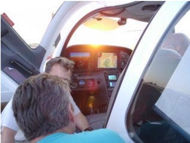
Of course, a favorite game amongst pilots is trying to make the cost of the instrument panel equal to or greater than the cost forward of the firewall. To this end, this aircraft is fitted not only with dual Garmin GNS-430s (more than I care to spend), but also with a large primary
