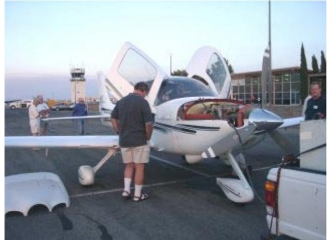
The Cirrus with the hood (*or bonnet*) off and the gull wing doors open. The aircraft is currently running off of a NTPS external power cart, which is basically a bunch of batteries in a box in the back of **Wen Painter's** pickup.
