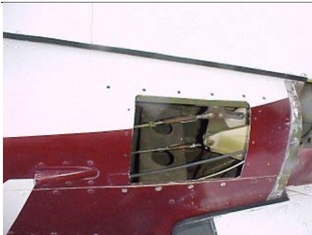
Completed access hole on left (port) side
