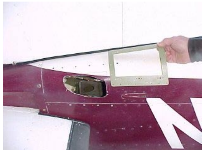
Opening up the hole to match the provided doubler
