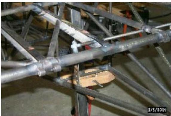
**Trim tab horn and torque tube**
