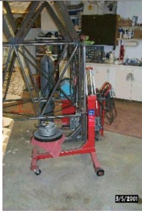
**Right side, looking left – car engine stand with “L” bracket with approximately 150 pounds to counter balance the weight of the fuselage and center section. When the wings are detached, this stand along with the one on the tail allows the fuselage to be rotated +/- 90 degrees from vertical. One person can rotate the fuselage with one hand in about 10 – 30 seconds.**
