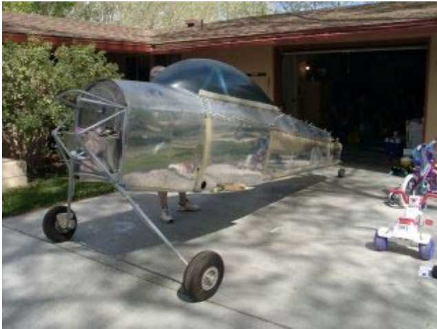
RV-4 fuselage with canopy installed
